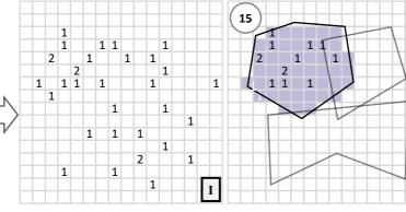
I. Render Points: Aggregate points within each pixel, and store result in pixel color channels.
