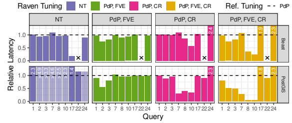
Figure 3: Cumulative benefit of tuning strategies for a representative query subset. NT: No Tuning, PdP: Projection Pushdown, FVE: Filter Vector Early, CR: Clip Raster. Baseline: PdP. Transparent: lower bounds on timeouts (>1000 sec).
